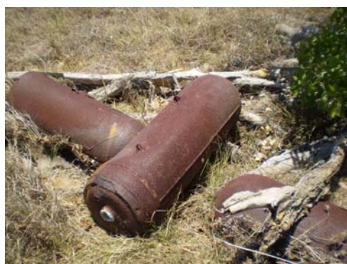
Heavily corroded WWII light case chemical bombs (500lb and 250lb) of UK origin discovered while clearing exDefence property in Queensland. Photograph courtesy of the Department of Defence
