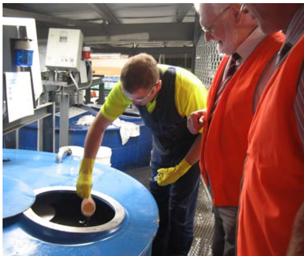
Site representative removing a chemical sample from the reaction vessel for analysis by OPCW inspectors.
