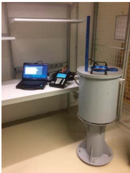
Prototype detector for solid waste measurement: (a) external view; (b) during performance testing (Images courtesy IAEA)
