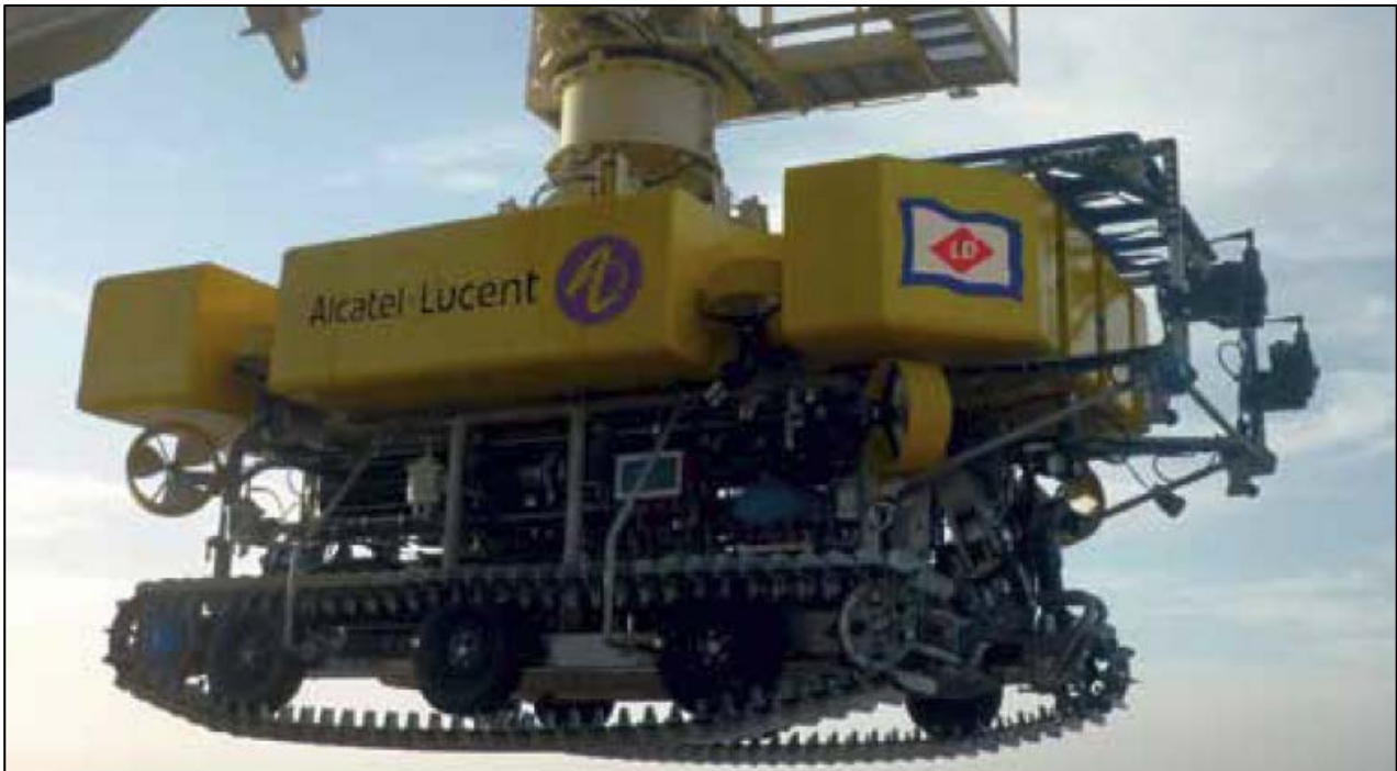
Figure 2-4. Example image of a Remotely Operated Vehicle being deployed from a cable ship.
