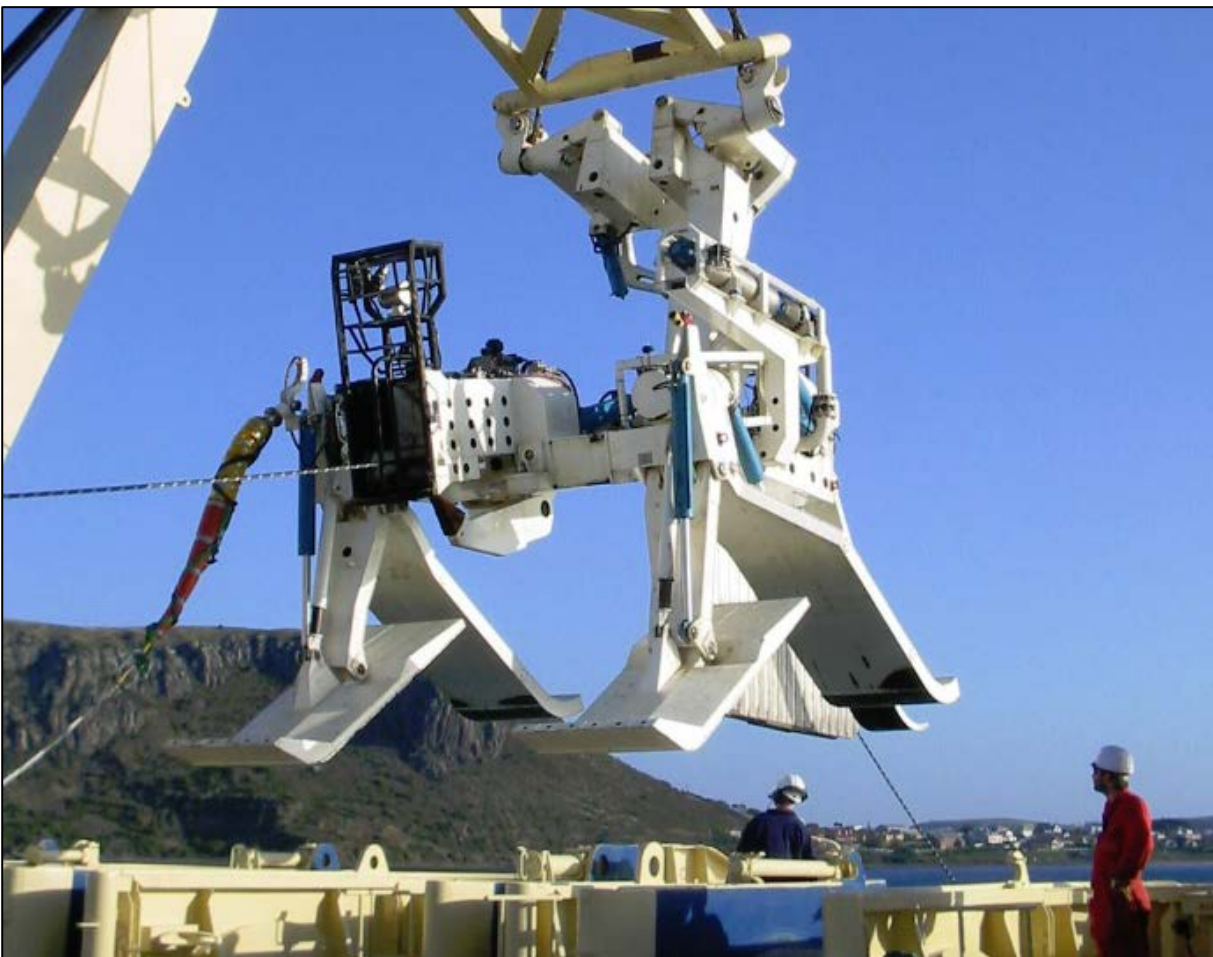
Figure 2-3. Example image of a cable plough on a cable ship.
