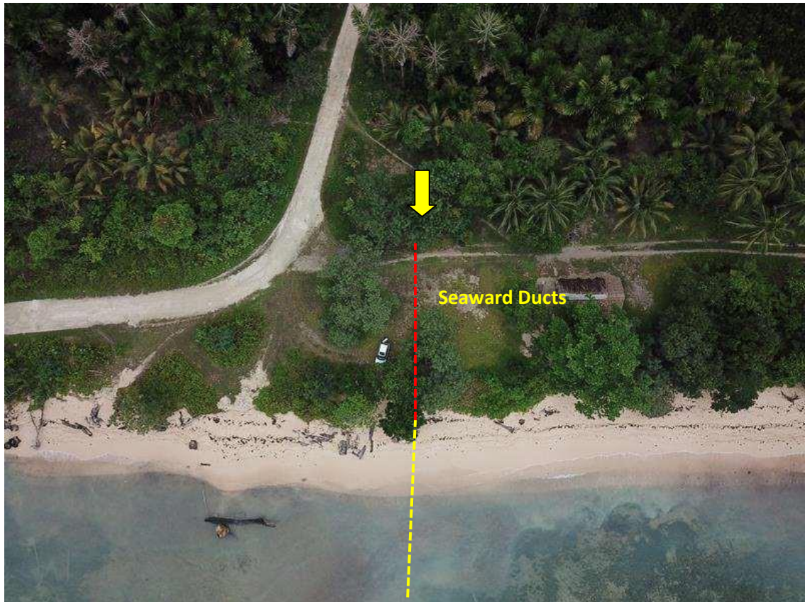
Figure 2-11 Auki BMH and proposed seaward ducts
